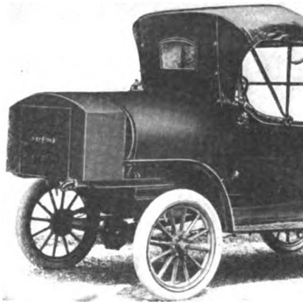
Q. D. gasoline delivery tank for Fords
